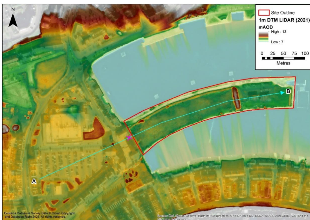
Figure 2-2 Site topography using Welsh Government's 2021 1m DTM LiDAR
