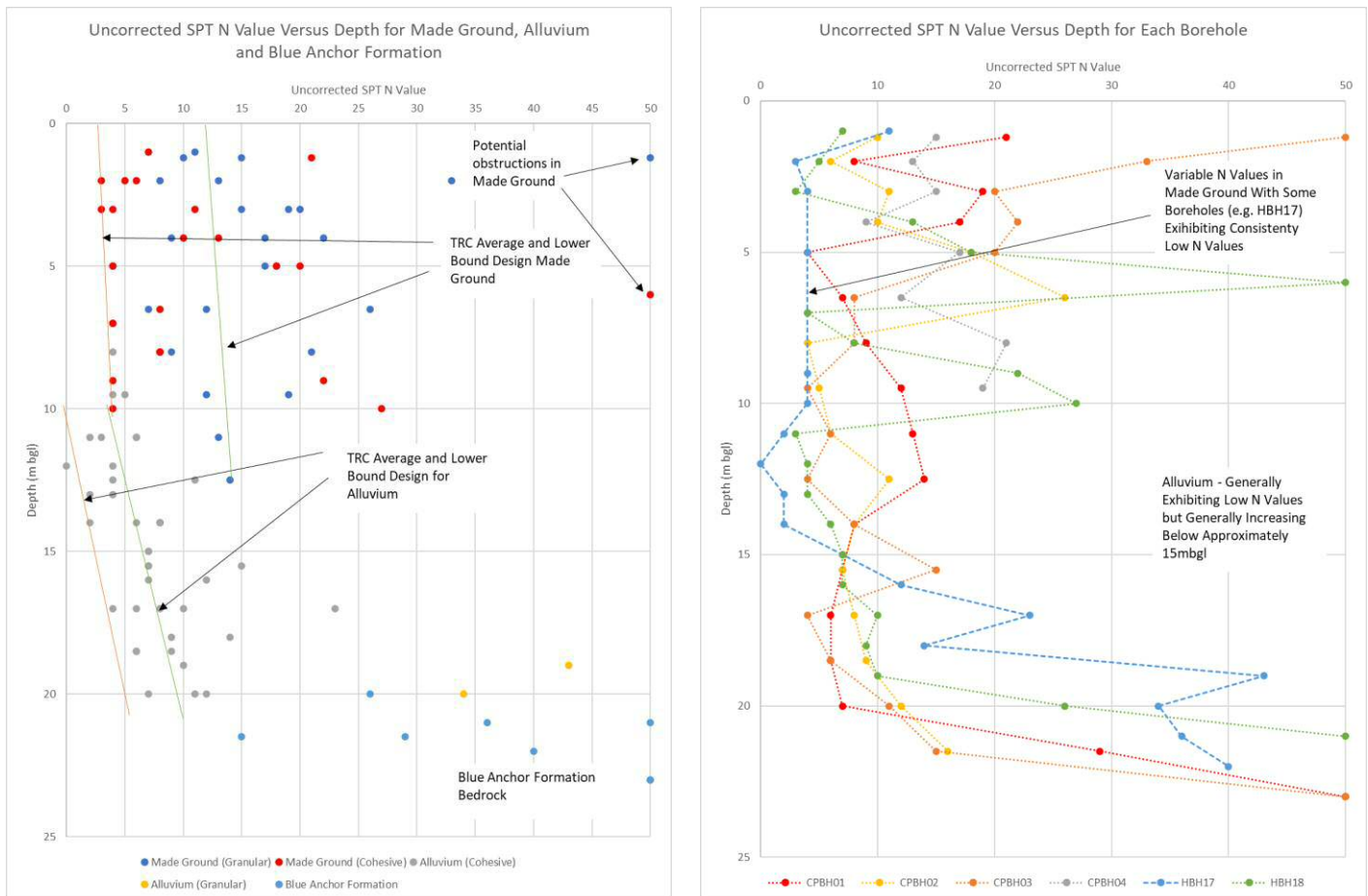
Figures 9 and 10: Uncorrected SPT N Value Versus Depth for Different Material Types and for Each Borehole
