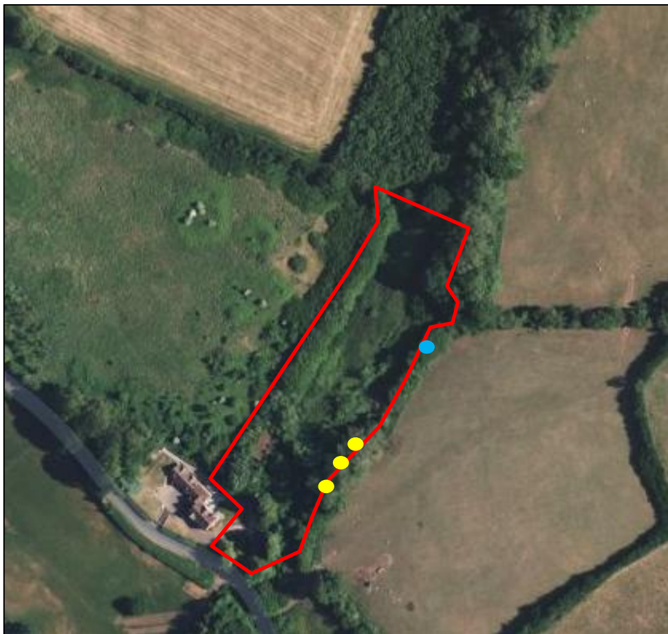
The plan above shows the location of the trees to be removed (large Ash trees shown coloured in yellow, the Ash tree with the large cavity is shown by the blue dot)
