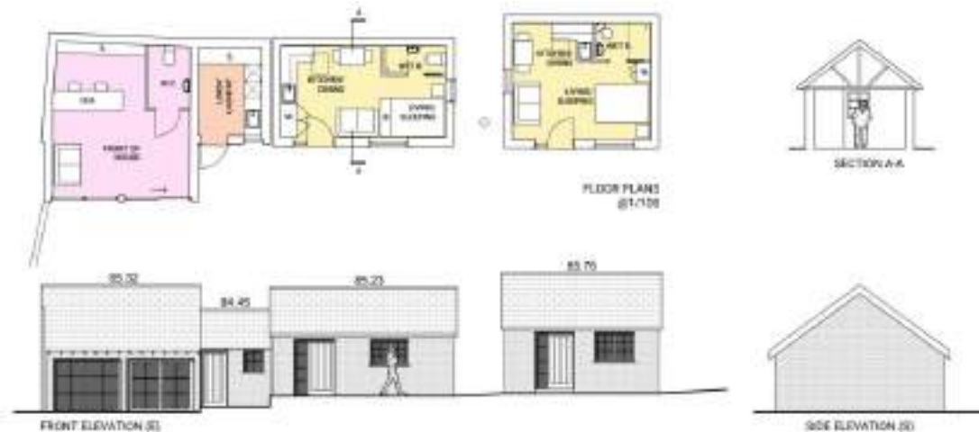
Proposed Plans and Elevations of Converted Buildings
