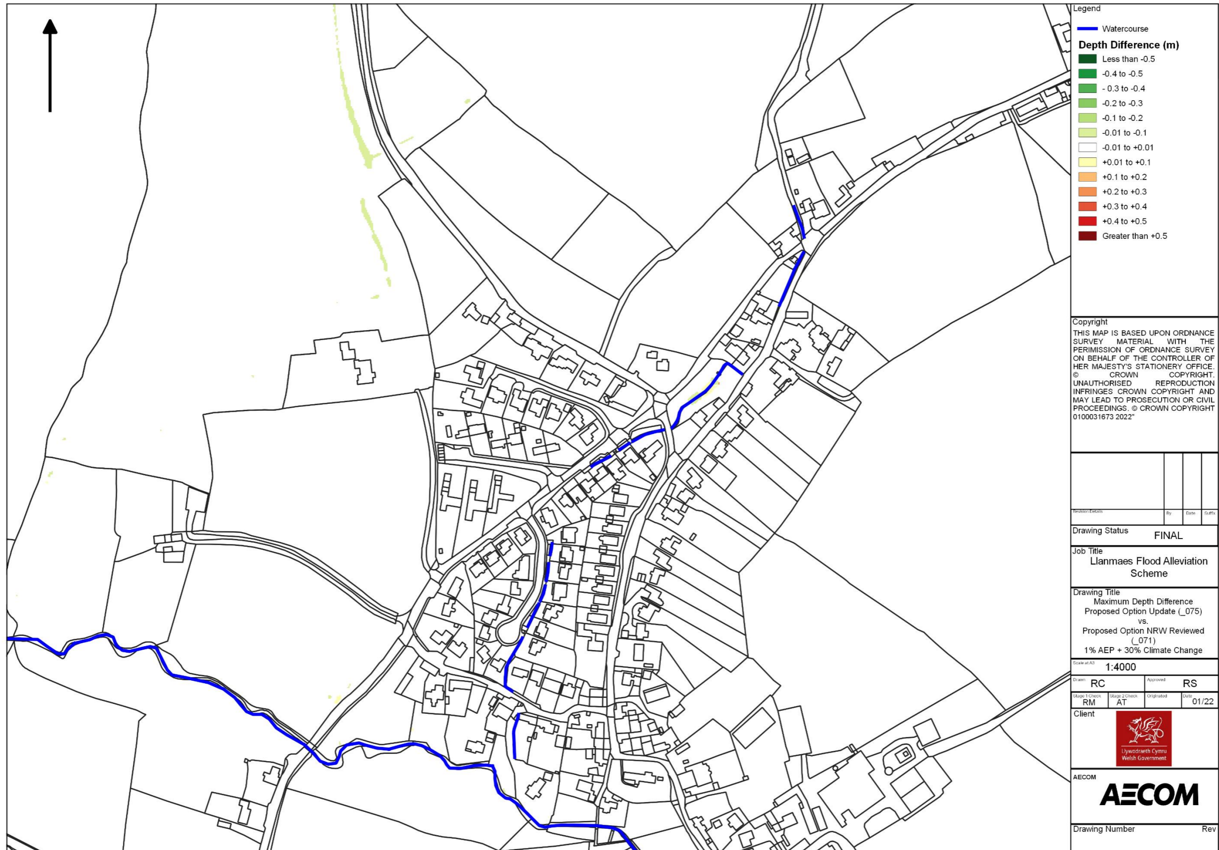
Figure 3-1: Maximum Depth Difference Plot, Llanmaes, 1% + 30%CC, Updated Proposed Option vs NRW Reviewed Proposed Option
