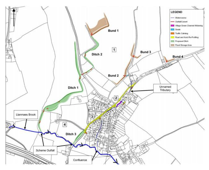
The proposed development is described in the submissions as being a low-impact 'soft' engineering solution. The scheme promotes the use of soft features such as flood bunds, ditches and swales to better manage the water flows naturally. In terms of materials management, all materials that would be excavated from the ditches and swales would be re-used on site to construct the flood bunds. The following aspects of the development are highlighted:
