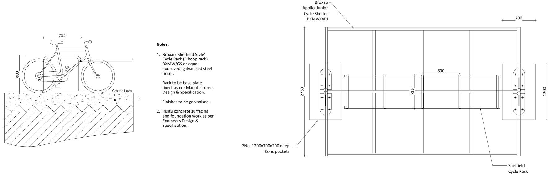
Cycle Rack Detail Side Elevation
