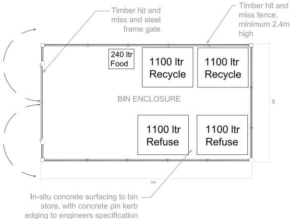
Bin Enclosure - Plan View Scale- 1:50
