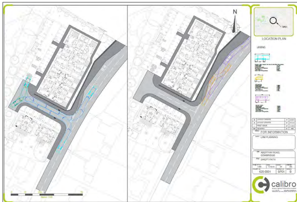
Figure 2-3 - Swept Path Analysis of Refuse Vehicle
