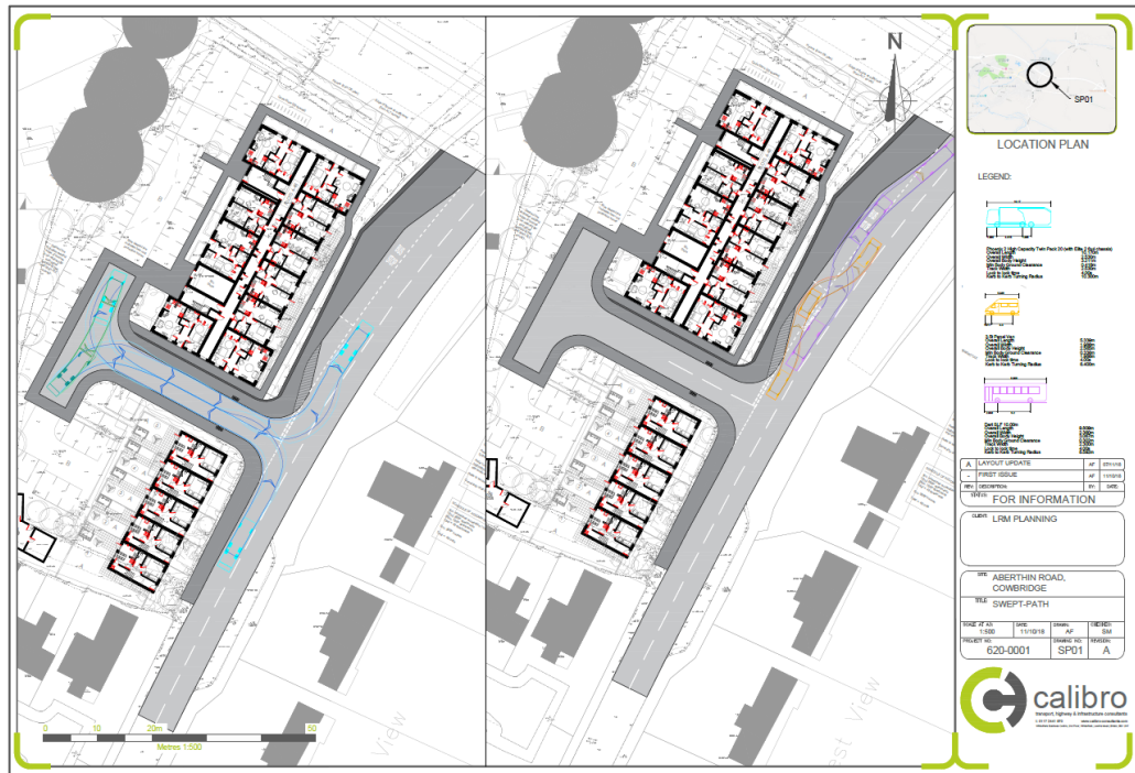
Figure 2-3 - Swept Path Analysis of Refuse Vehicle
