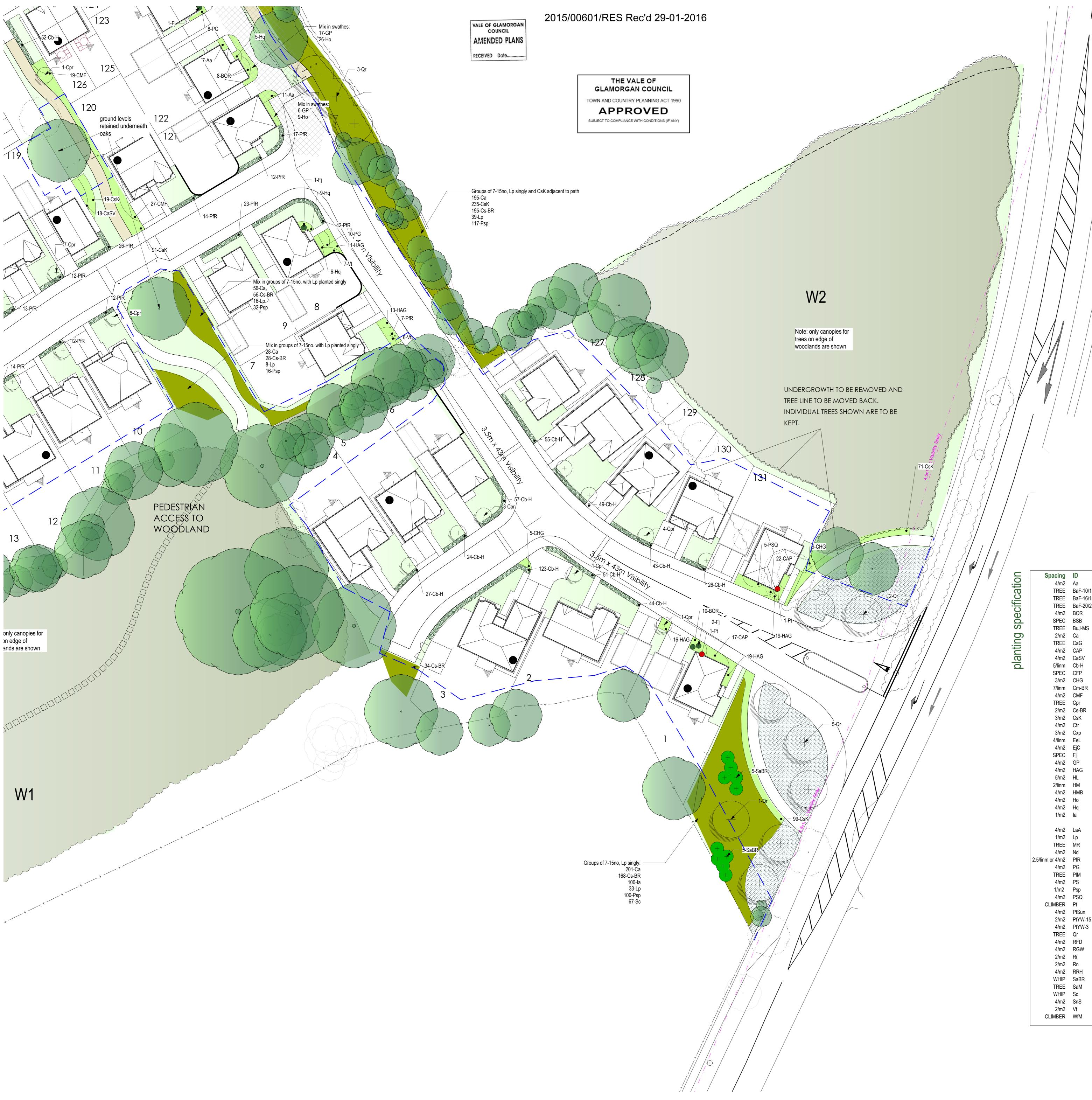
Tree locations are subject to confirmation of engineering and foundation details. Foundations shall comply with guidelines set by structural engineering consultants, and shall accord with the current NHBC Standards 'Building near Trees' and shall accommodate immediate and future impact of • Tree pits to be excavated to minimum 1m x 1m x
