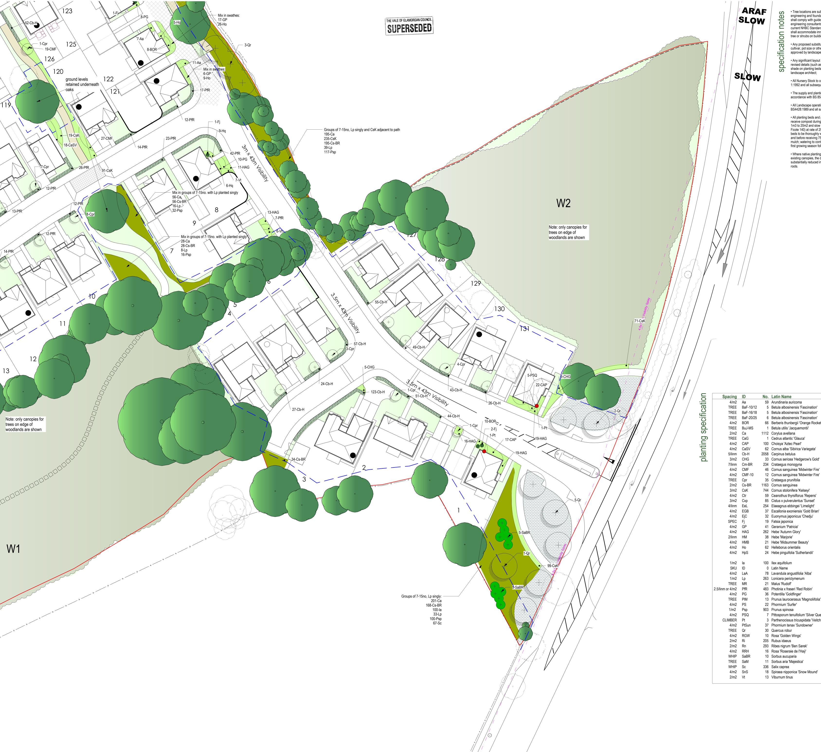
Tree locations are subject to confirmation of engineering and foundation details. Foundations shall comply with guidelines set by structural with Greenleaf 'Root Rain Urban' watering pipes, engineering consultants, and shall accord with the current NHBC Standards 'Building near Trees' and
