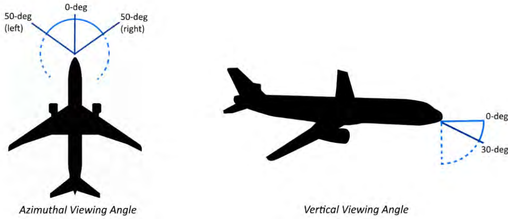
Figure 8 Aircraft field-of-view defined by azimuthal and vertical viewing angle parameters
