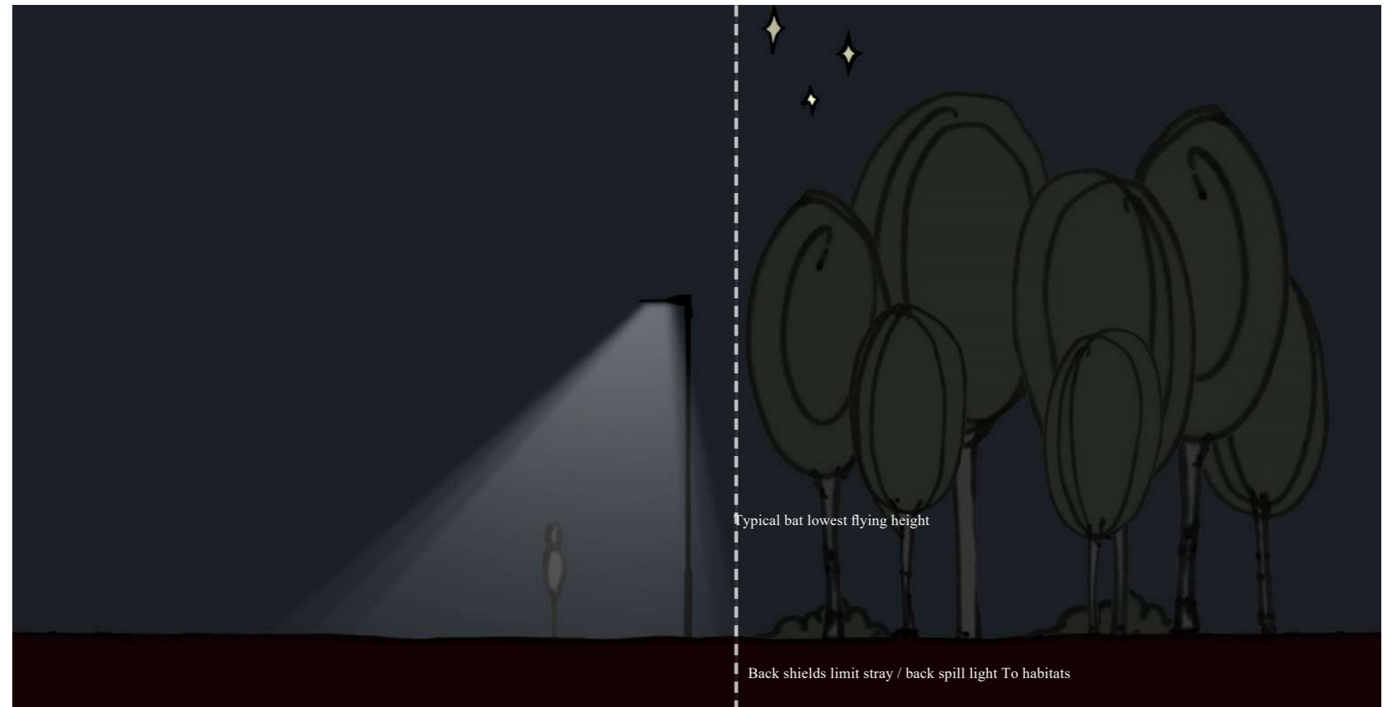
Figure 22: Use of back shields to prevent stray light to woodland areas
