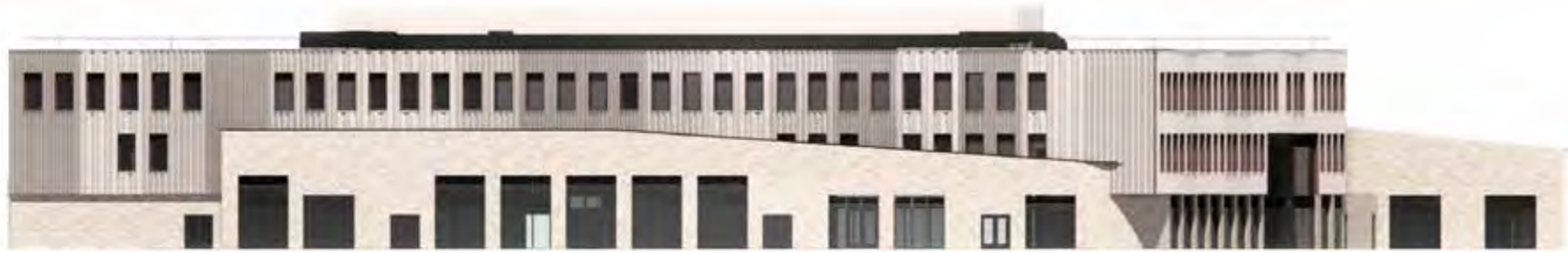
Option 2: Parapet line falls from the end of the double height spaces
