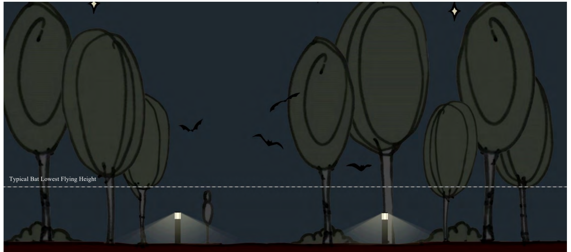
Figure 40: Low-level luminaire with no direct upward light emission
