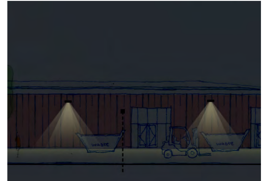
Figure 10: Lighting concept - service & storage yards
