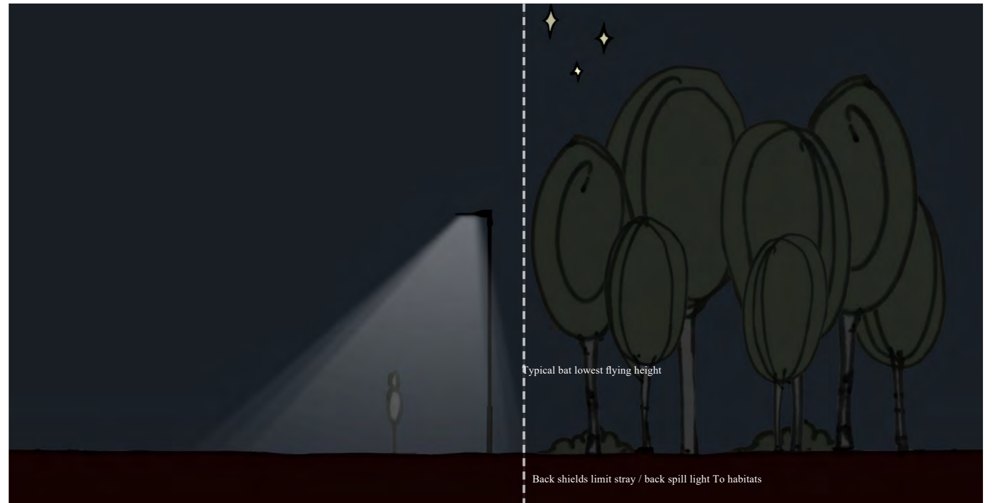
Figure 36: Use of back shields to prevent stray light to woodland areas
