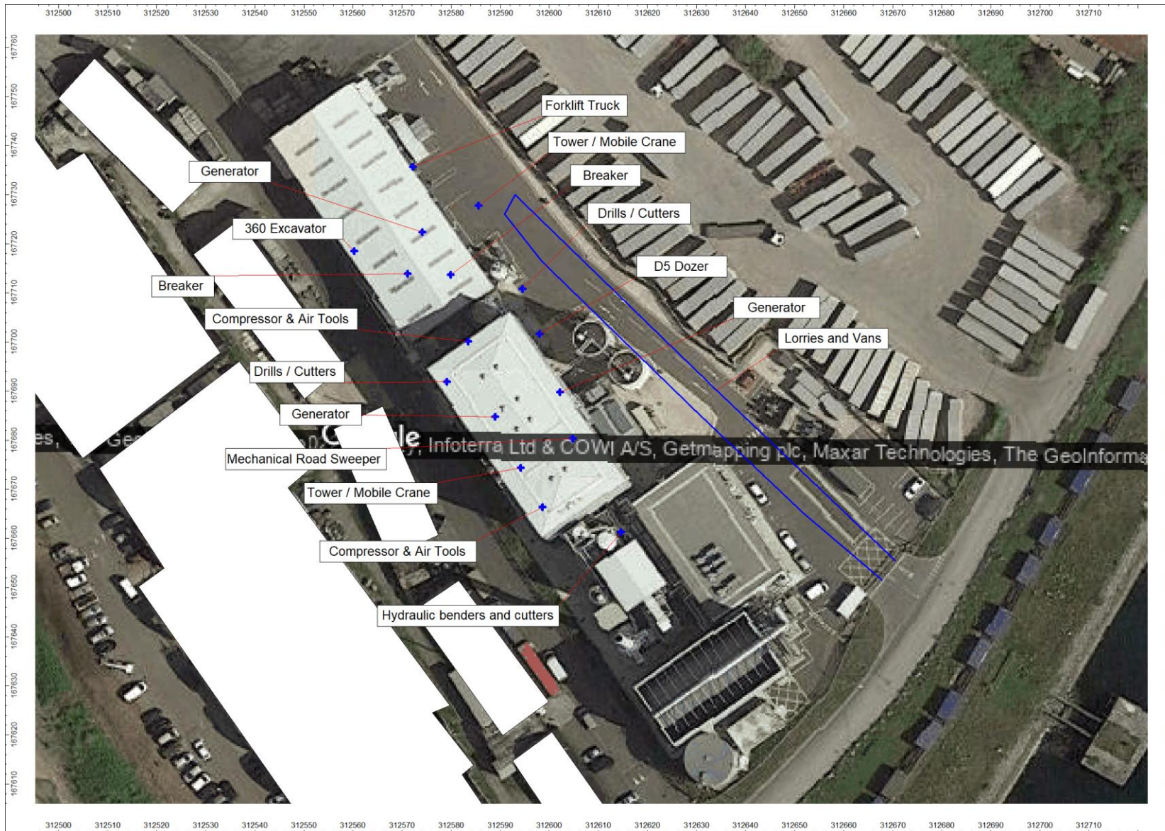
Figure A8.5.6: Site plan indicating grid coordinate references x, y coordinates for all external noise sources for the Decommissioning Phase
