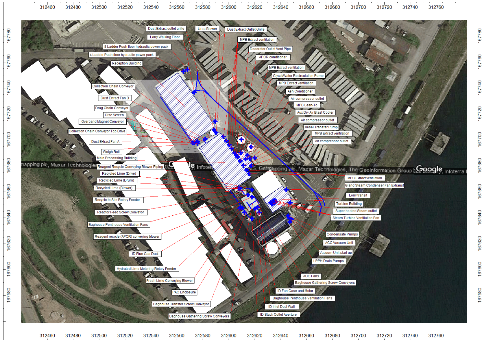
Figure A8.5.5: Site plan indicating grid coordinate references x, y coordinates for all external noise sources for the Operational Phase
