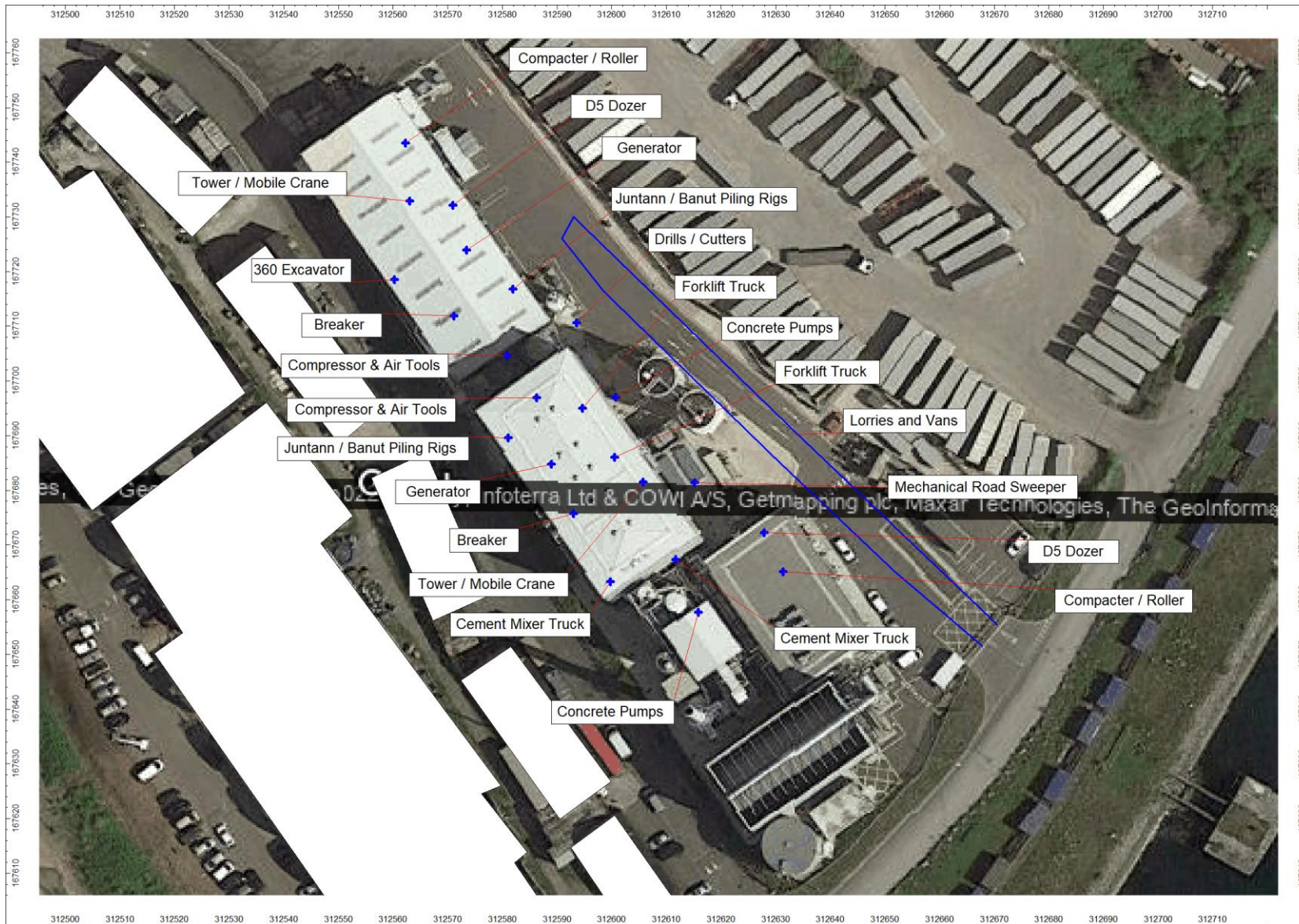
Figure A8.5.3: Site plan indicating grid coordinate references x, y coordinates for all external noise sources for Stage 3 of the Construction Phase
