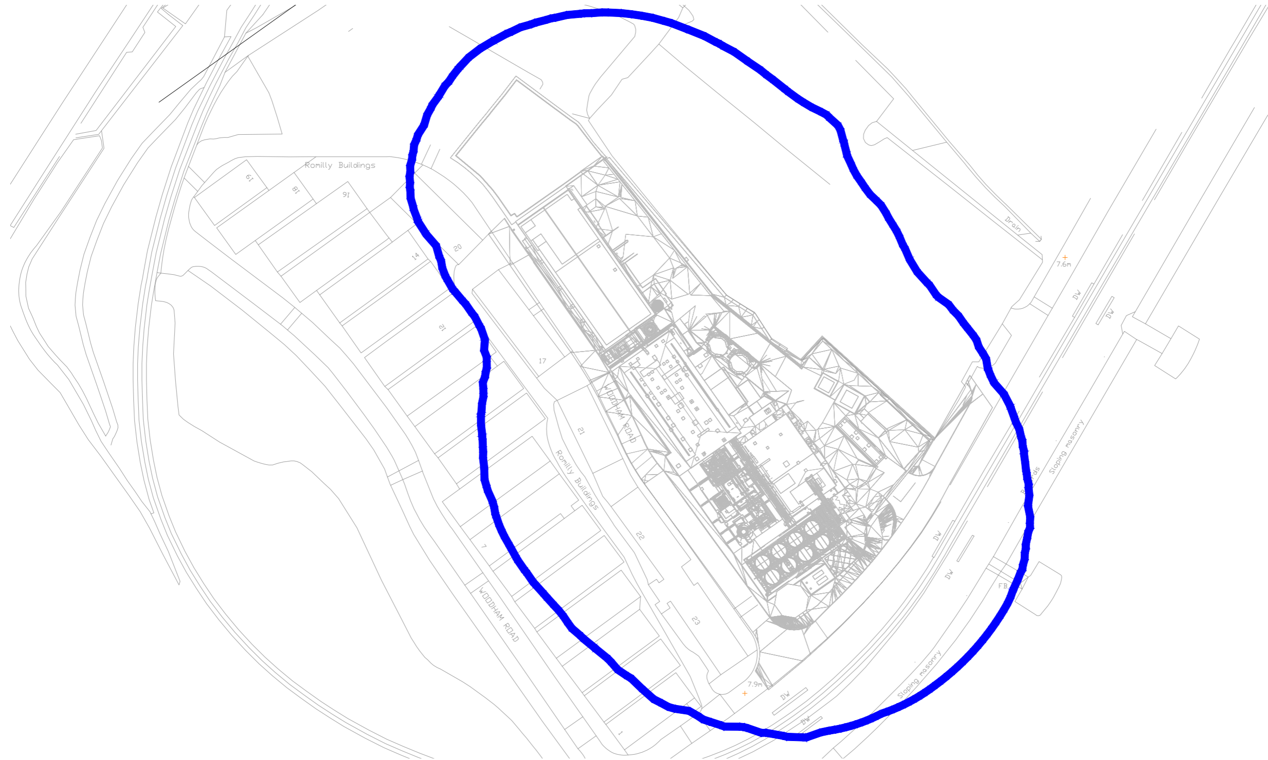
Figure 3.4. Image taken from drawing supplied - Showing 0.5 lux Isoline horizontal light levels at ground level.
