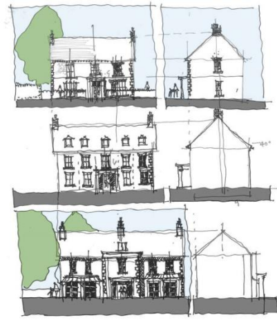
Sketch Facade Treatment - Option 3 (not to scale) Classically proportioned and detailed dwellings using stone and render
