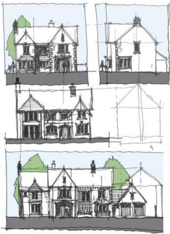
Sketch Facade Treatment - Option 1 (not to scale) Use traditional icons based on a 'rectory/revival' aesthetic
