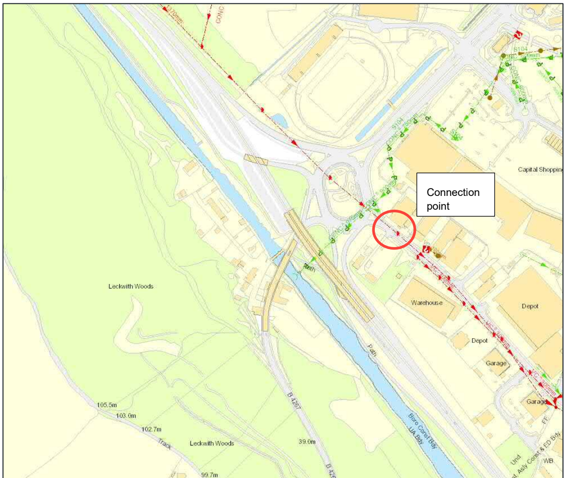
Figure 3-1 – Foul Connection Points
