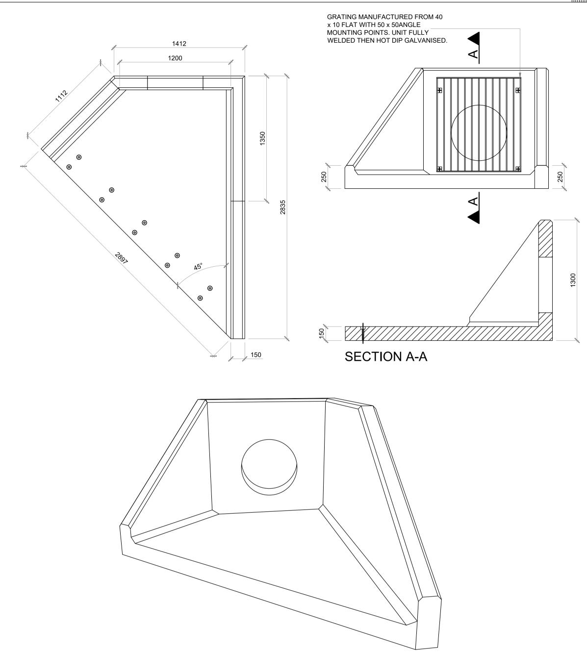
ALTHON AH12CA RH HEADWALL CLOSE COUPLED GRATING **SCALE 1:20**
