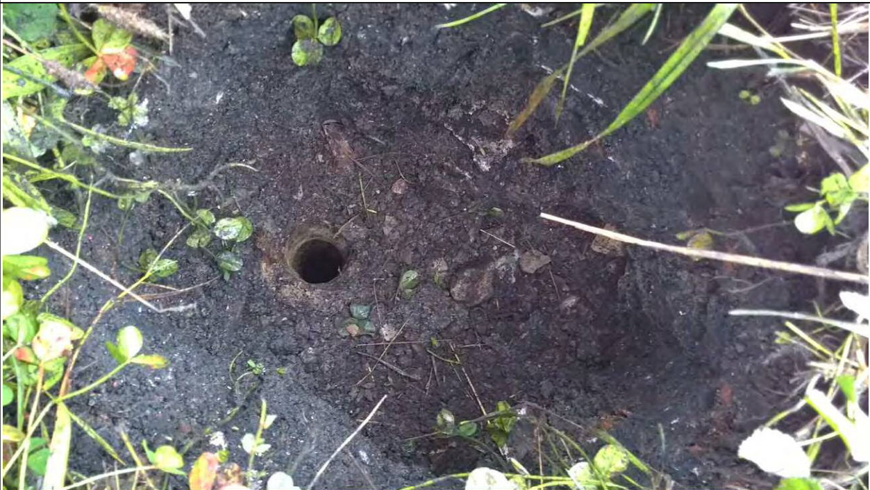
(WS04 0.4 m with SPT into bedrock)
