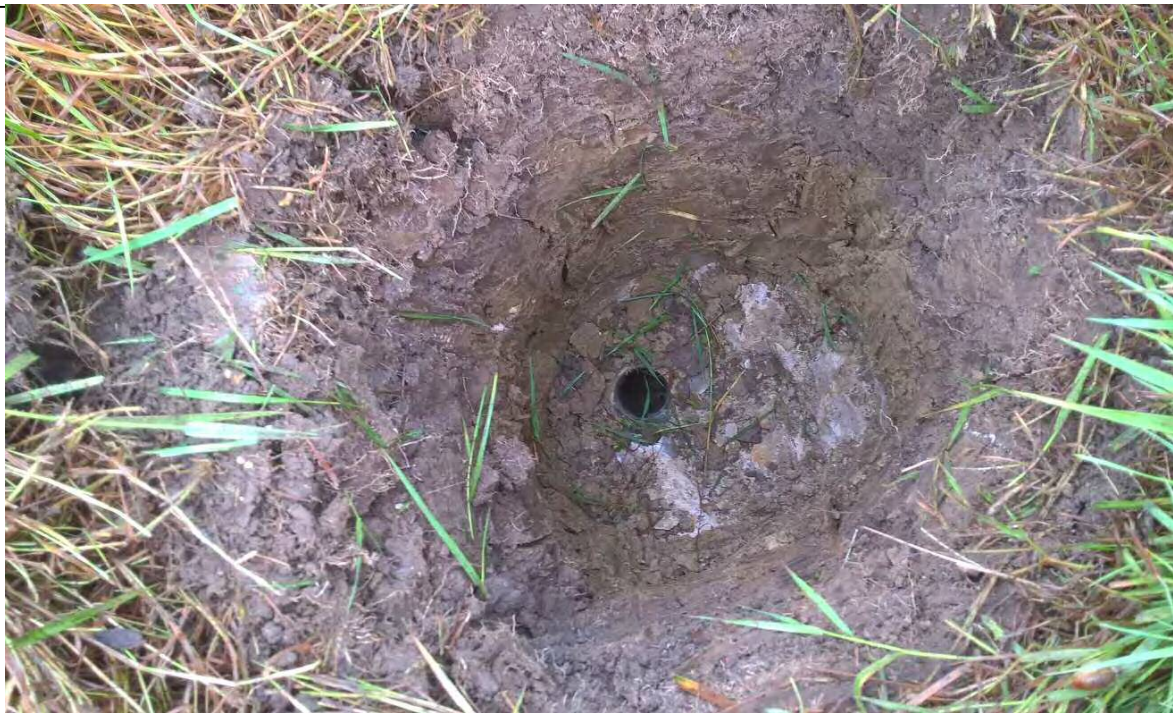
(WS06 0.6 m with SPT into bedrock)
