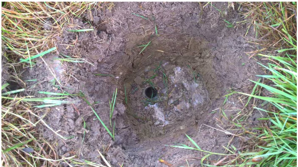
(WS05 0.6 m with SPT into bedrock)
