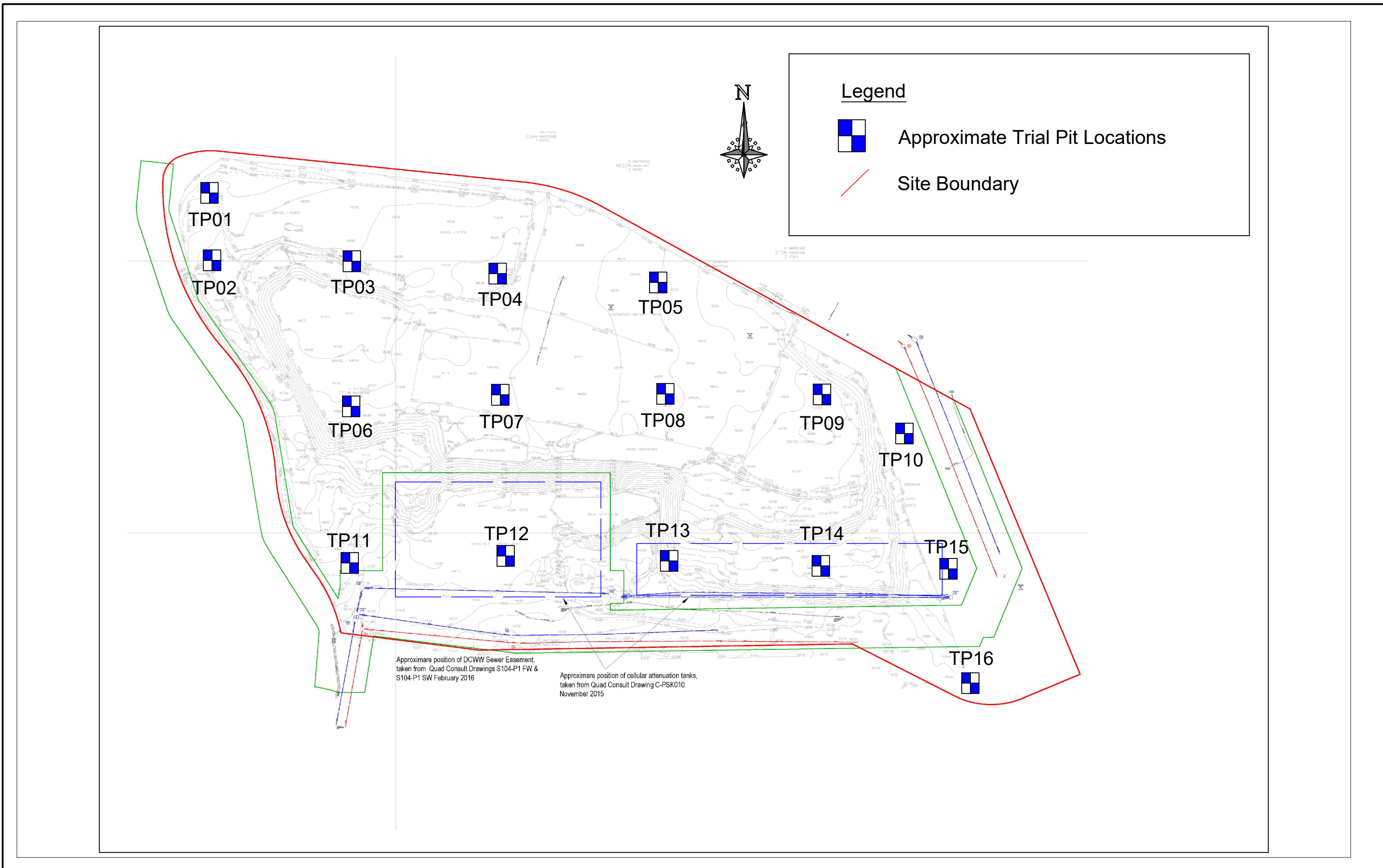
Figure 1: Grid Sampling Locations Project: Llancarfan Primary School Job No.: 12658 Intégral Géotechnique Integral House, 7 Beddau Way, Castlegate Business Park, Caerphilly, CF83 2AX. Tel: 029 2080 7991 Client: Taylor Wimpey South Wales Scale: NTS
