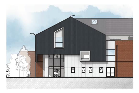
Notwithstanding the generally traditional form, the proposed materials are contemporary and they would elevate the appearance of the building. The main part of the elevations and the roof would be finished in a metal cladding and the ground floor (and other feature elements) would be brick. The plans indicate grey windows and aluminium rainwater goods. It is considered that the high quality palette of materials will add positively to the character of the building and create visual interest.
