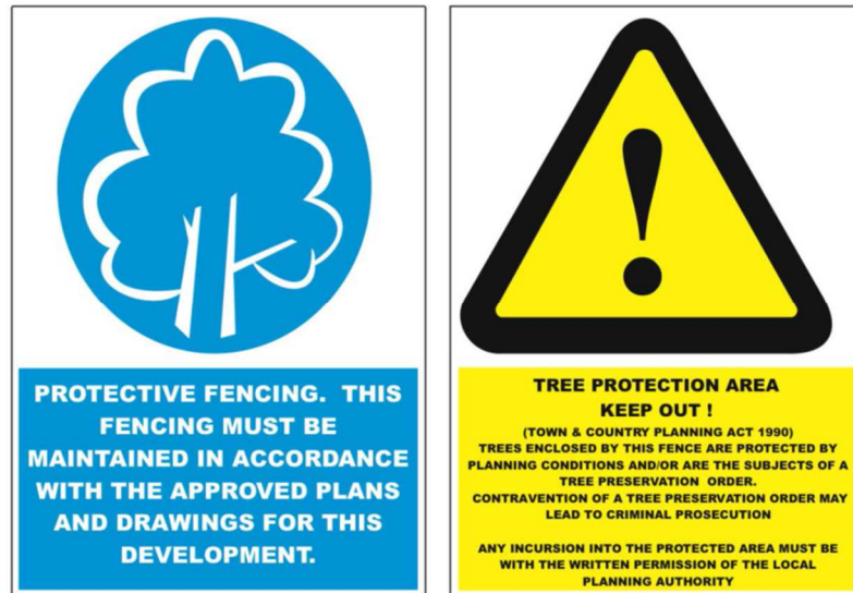
Figure 4: Tree Protection Signage
