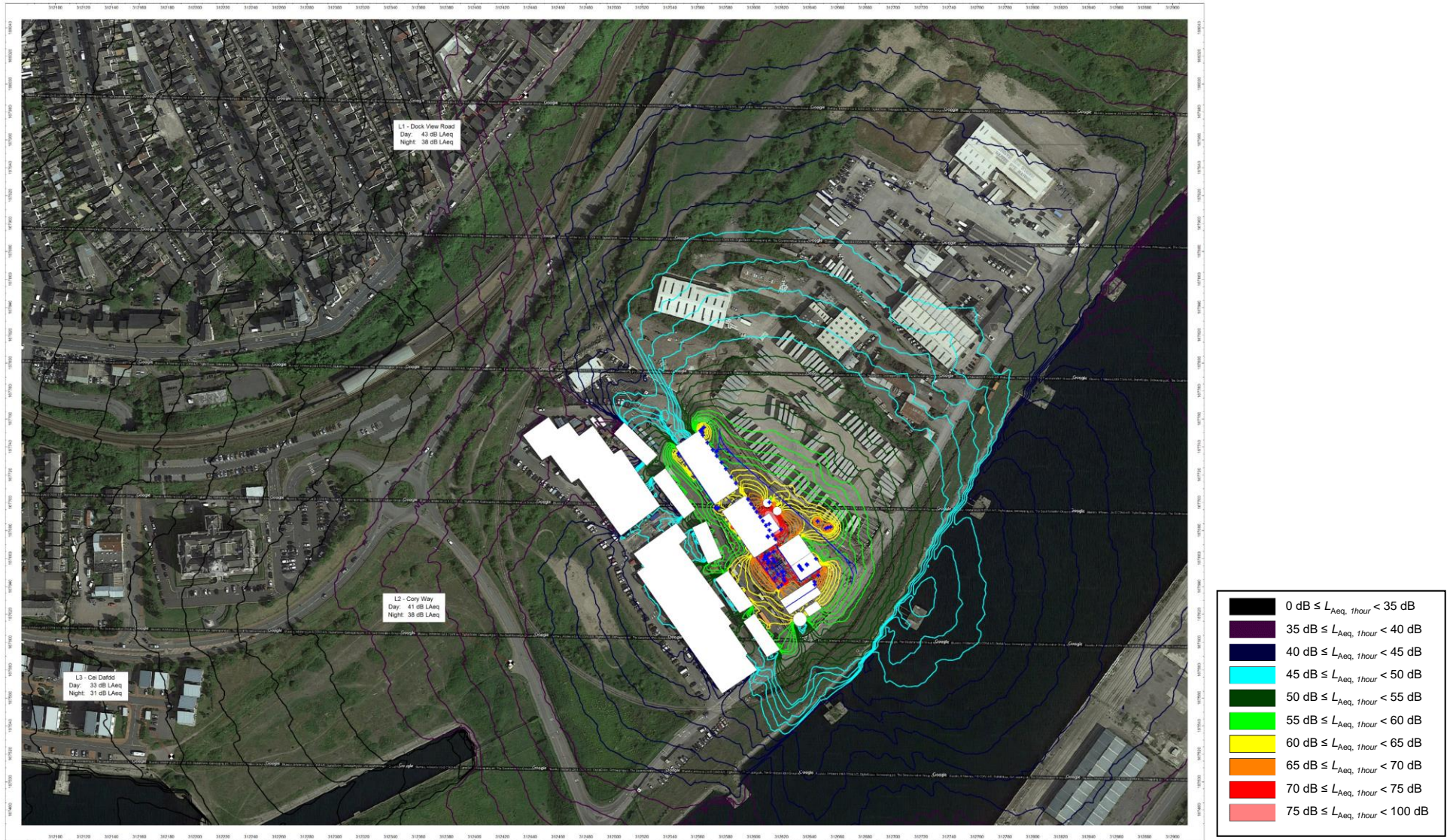
Figure D2: Predicted night-time L_{Aeq,15hour} noise level impact from the Site at 4.5m above local ground level
