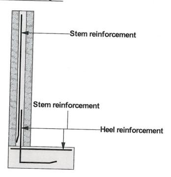
Heel mesh - A393 - (393 mm²/m) Stem mesh - A393 - (393 mm²/m)
