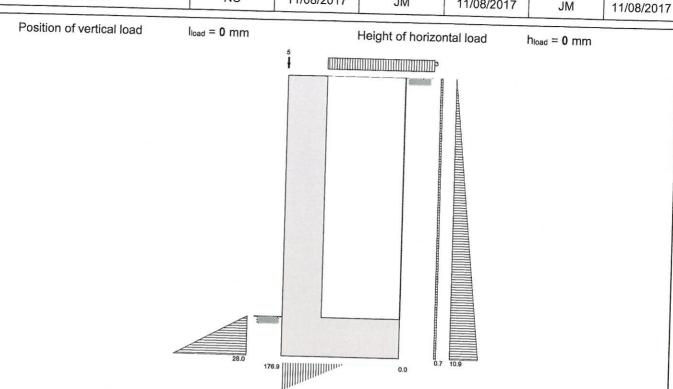
Loads shown in kN/m, pressures shown in kN/m<sup>2</sup>
