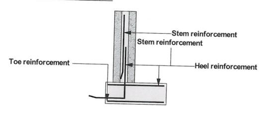
Toe mesh - A393 - (393 mm²/m) Heel mesh - A393 - (393 mm²/m) Stem mesh - A393 - (393 mm²/m)
