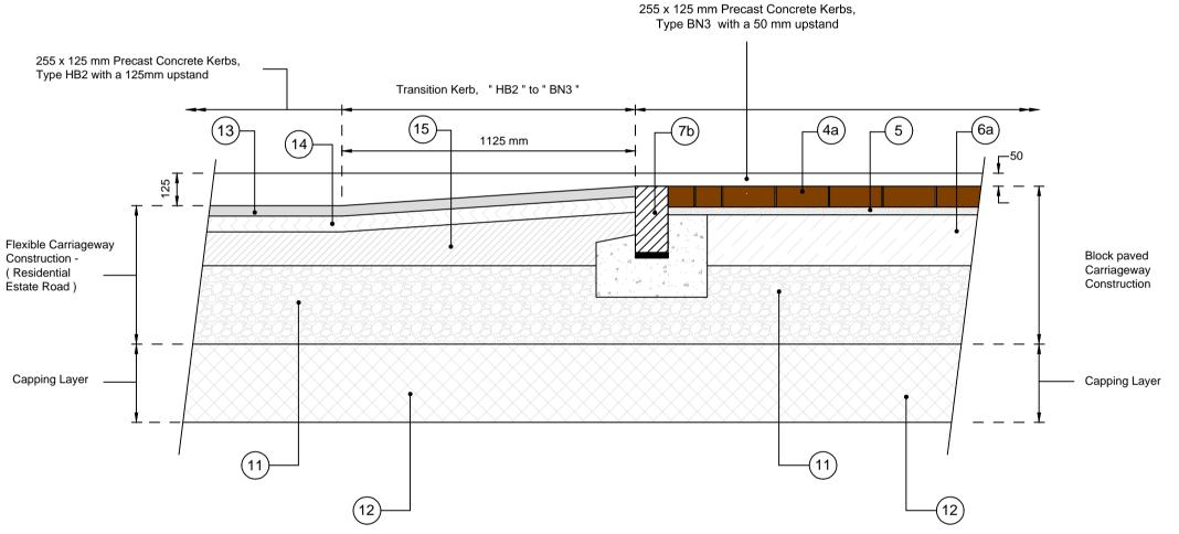
Section Through of Block Paved Raised Junction / Plateau Area incorporating Flexible carriageway / Ramp construction along Access Road -Max Ramp upstand 75mm
