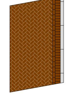
Concrete Block Paving, Colour "Red Brindle" laid in a 45 \* Herringbone Pattern within carriageway and 90 \* within Footway / Margin. (Location - Raised Junctions, Mews Court Construction) - Scale N.T.S
