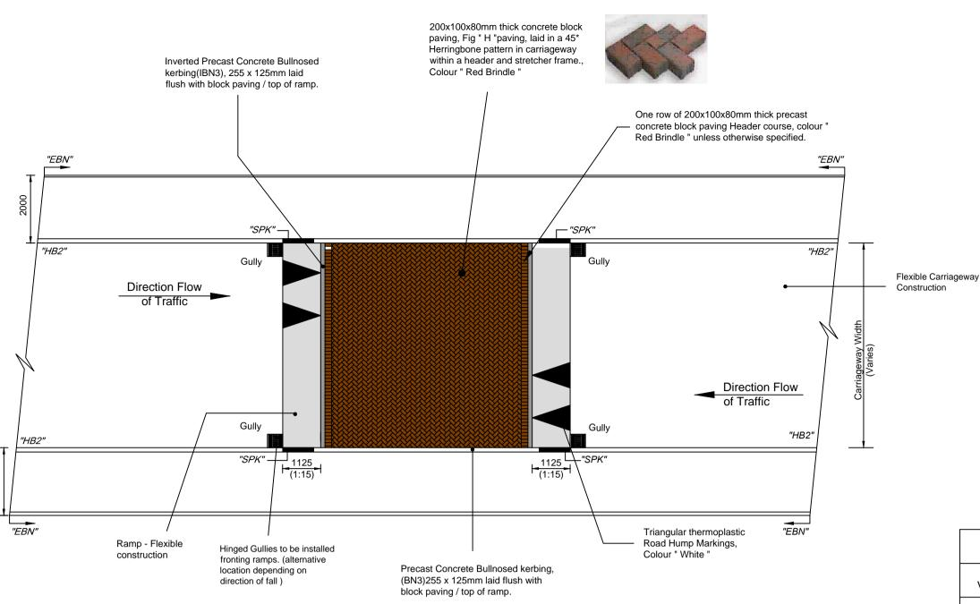
Plan View of Block Paved Raised Plateau Area incorporating Flexible Ramps and
