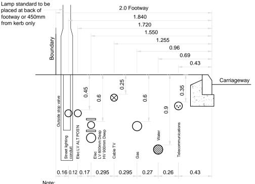
Not all services are expected to be within, or on the same, footway side. where the footway width is less than 2.0m the contractor shall seek guidance
