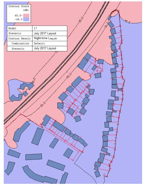
3131/NM2 – Night-time Comparison with 45dB LAeq,8hr Trigger Level (Ground Floor)
