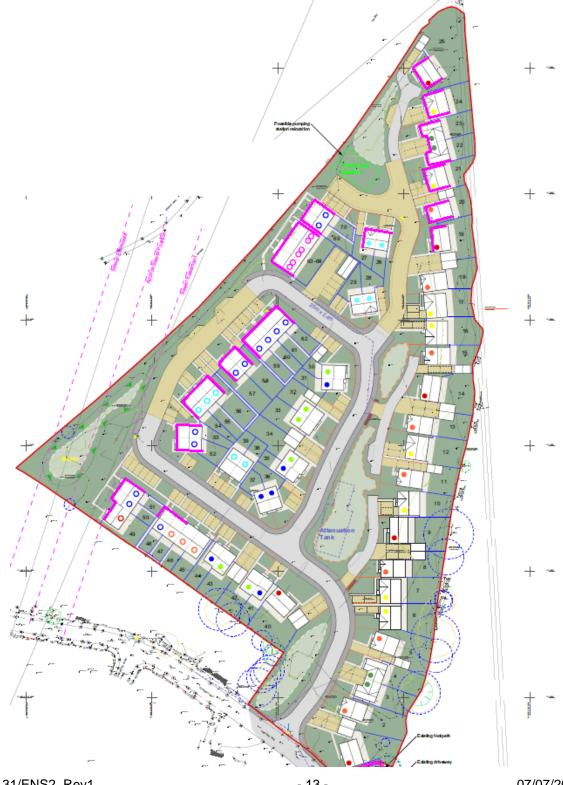
All <u>bedrooms</u> on the façades highlighted above in **PINK** require up-rated acoustic glazing and all habitable rooms require active ventilation units as specified below. Standard thermal double glazing should be sufficient on remaining habitable rooms.
