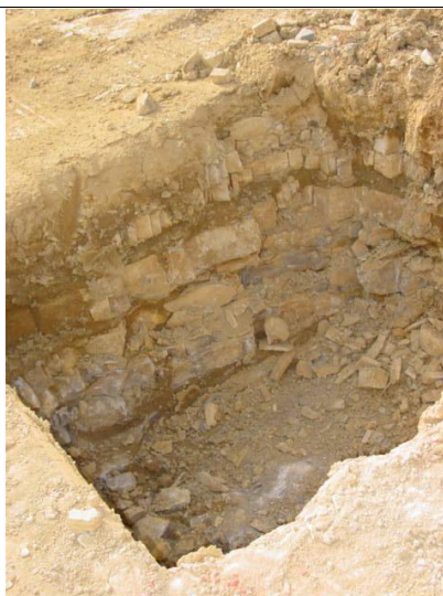
Plate 2: Photograph showing thin mudstone partings.
