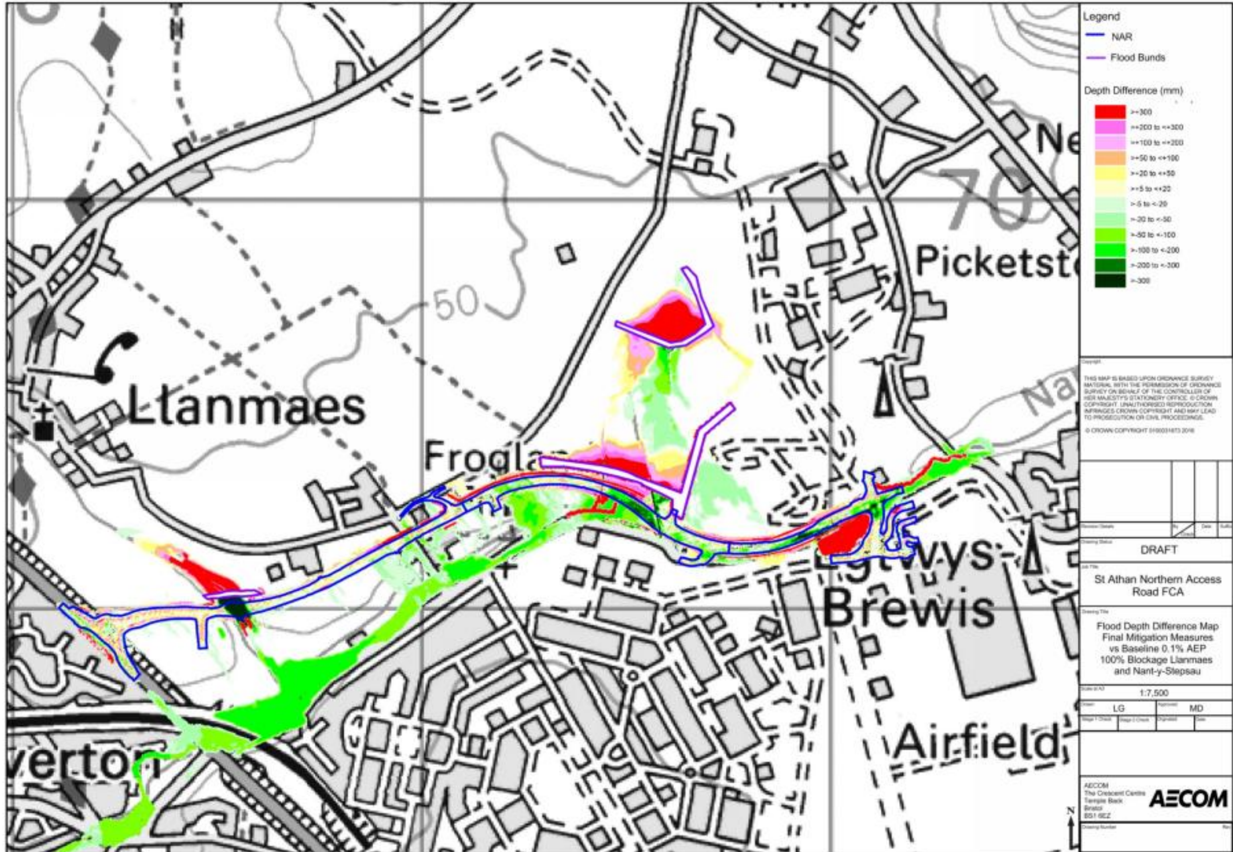
Figure 6-12 - Flood Depth Difference, 0.1% AEP + 100% Blockage of Llanmaes and Nant y Stepsau
