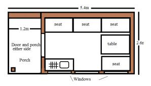
The moduLog Mawr is a moduLog made up of 3 modules plus a covered porch. There are many different designs possible using the 4 different moduLog modules.
