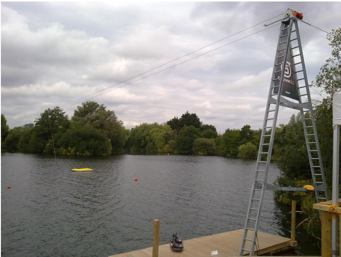
The start pylon on the Sesitec 2.0 cable system at JB Ski Wake Park in Surrey
