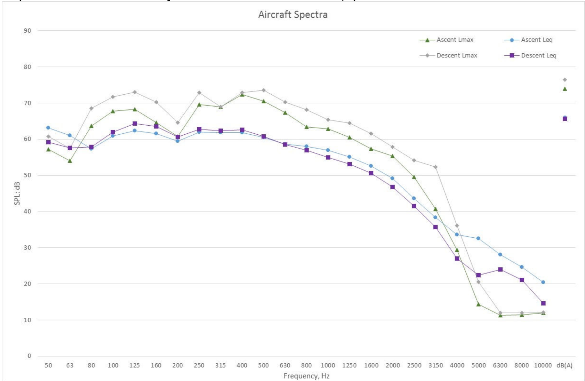
Graph 4365/G2 – Source Aircraft Flyover Third-Octave Band L Max and L eq Spectra at Position B
