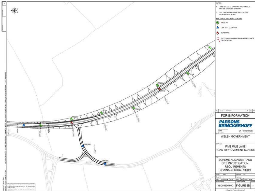
Figure 3: Location of Test Pits and Boreholes
