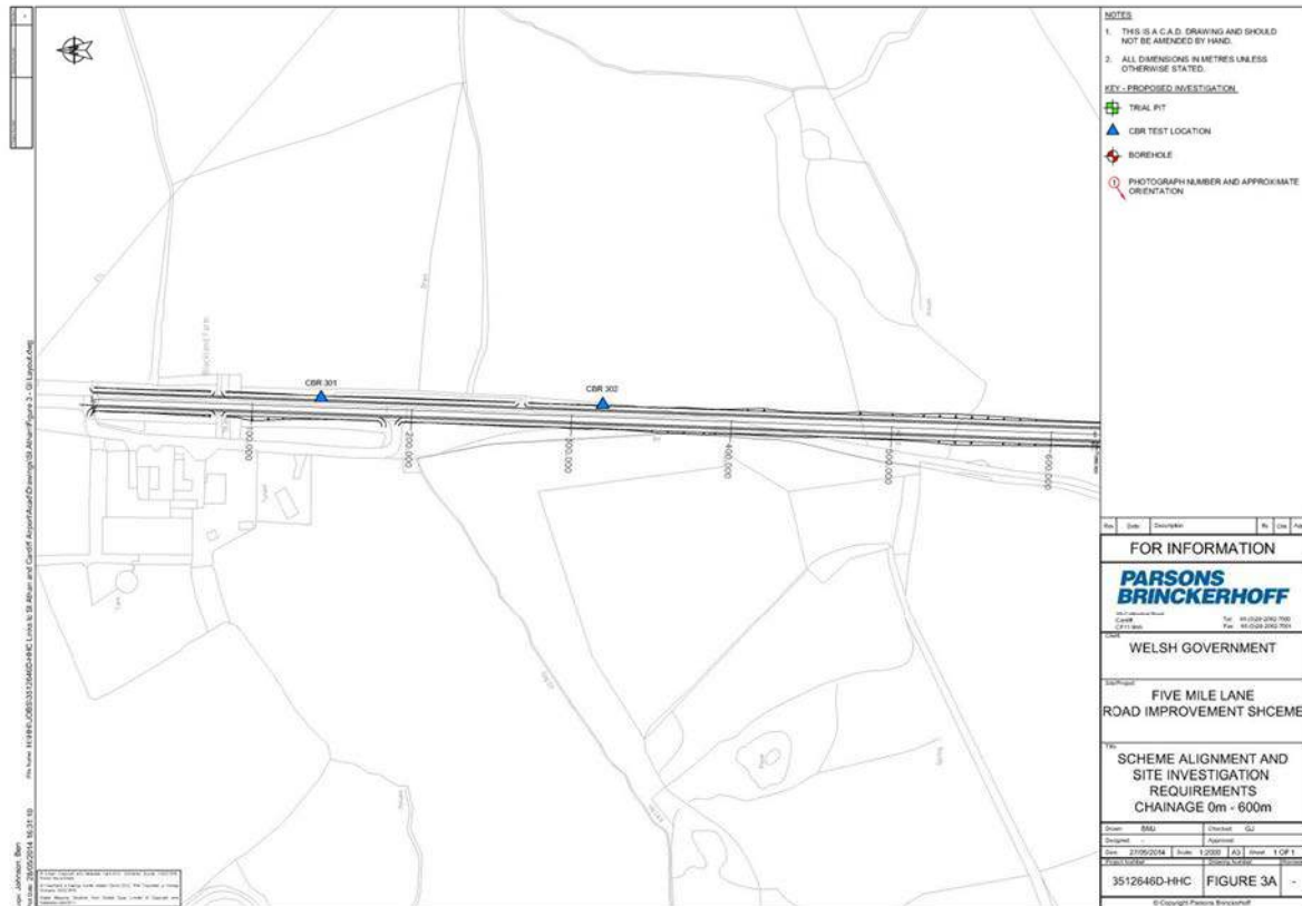
Figure 2: Location of Test Pits and Boreholes
