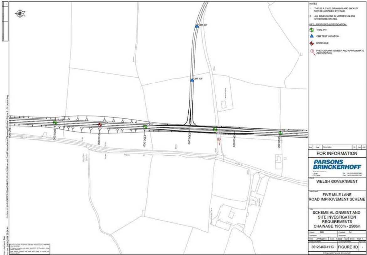
Figure 5: Location of Test Pits and Boreholes
