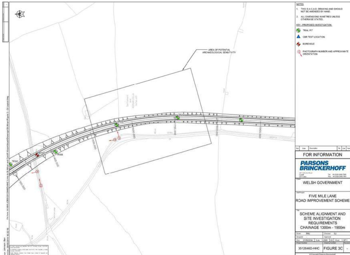
Figure 4: Location of Test Pits and Boreholes
