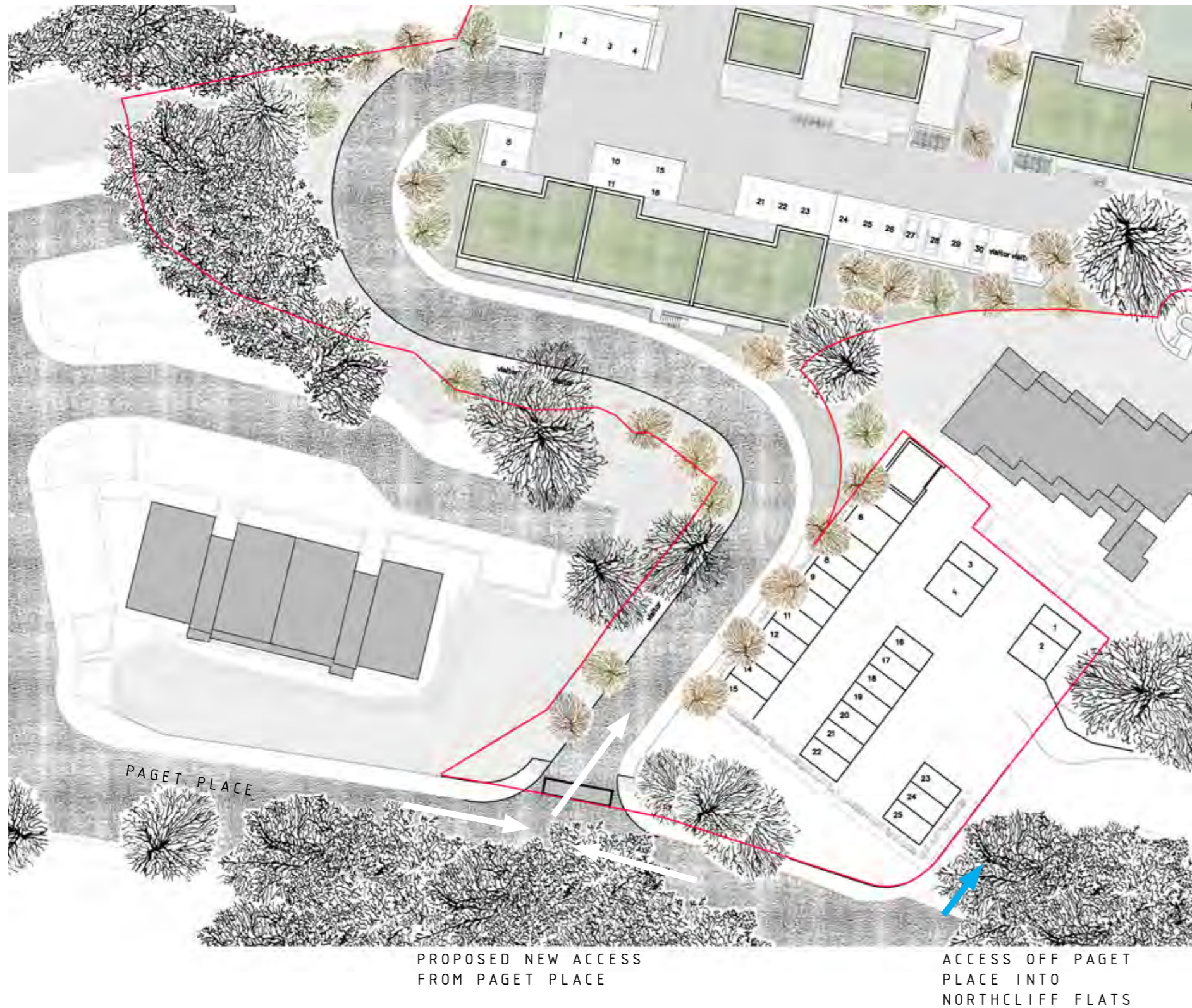
Above: A new access point off Paget Place is proposed to serve the potential development at Northcliff Lodge. The current access via Northcliff Drive would not be adequate in serving the development proposal.
