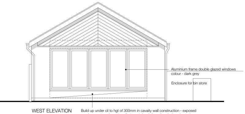
sand cement render exturnally to match existing - face below dpc to be in face brickwork to match existing - 60mm 'Kingspan'ridgid board insulation in cavity
