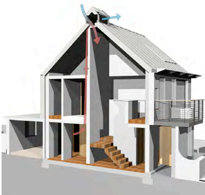
The principal of a heat recovery system means that warm air can be retained within the house thus minimising the heating requirements. In addition to this, along with an air tight fabric, it will moderate and control the air flow within the properties
