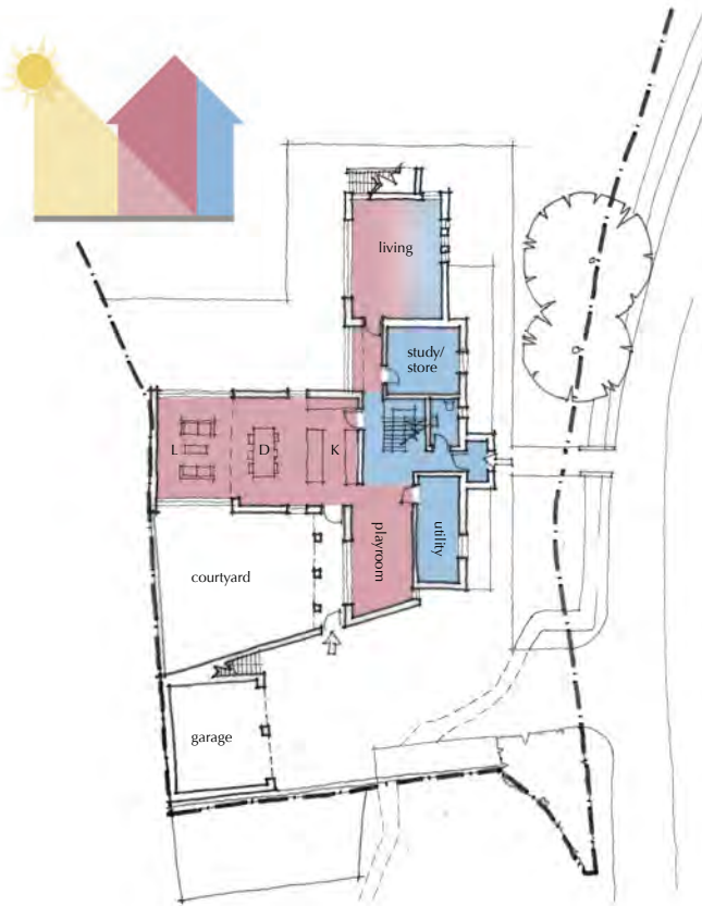
This earlier plan shows how room locations were considered during the design evolution to maximise access to sunlight
