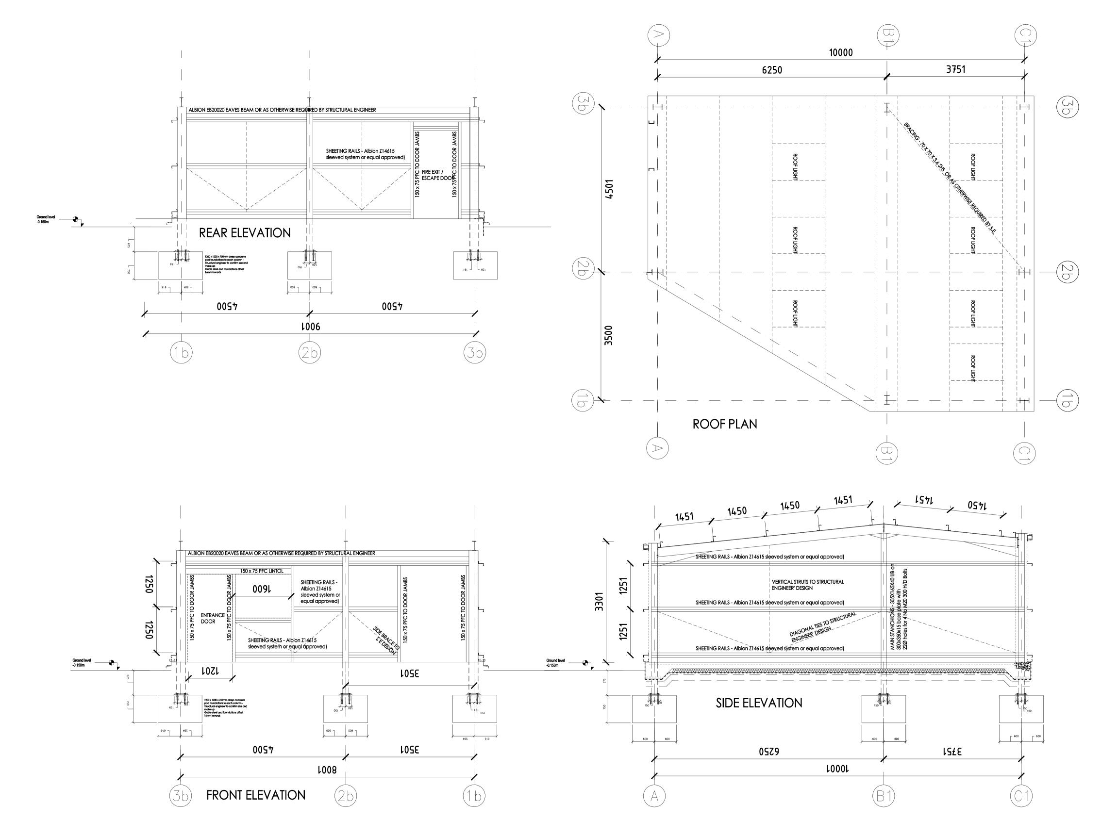
1200 X 1200 X 750mm deep mass concrEte pad foundations to each stanchion - all to Structural Engineer' specification and design Gable steel and foundations offset 16mm inwards
