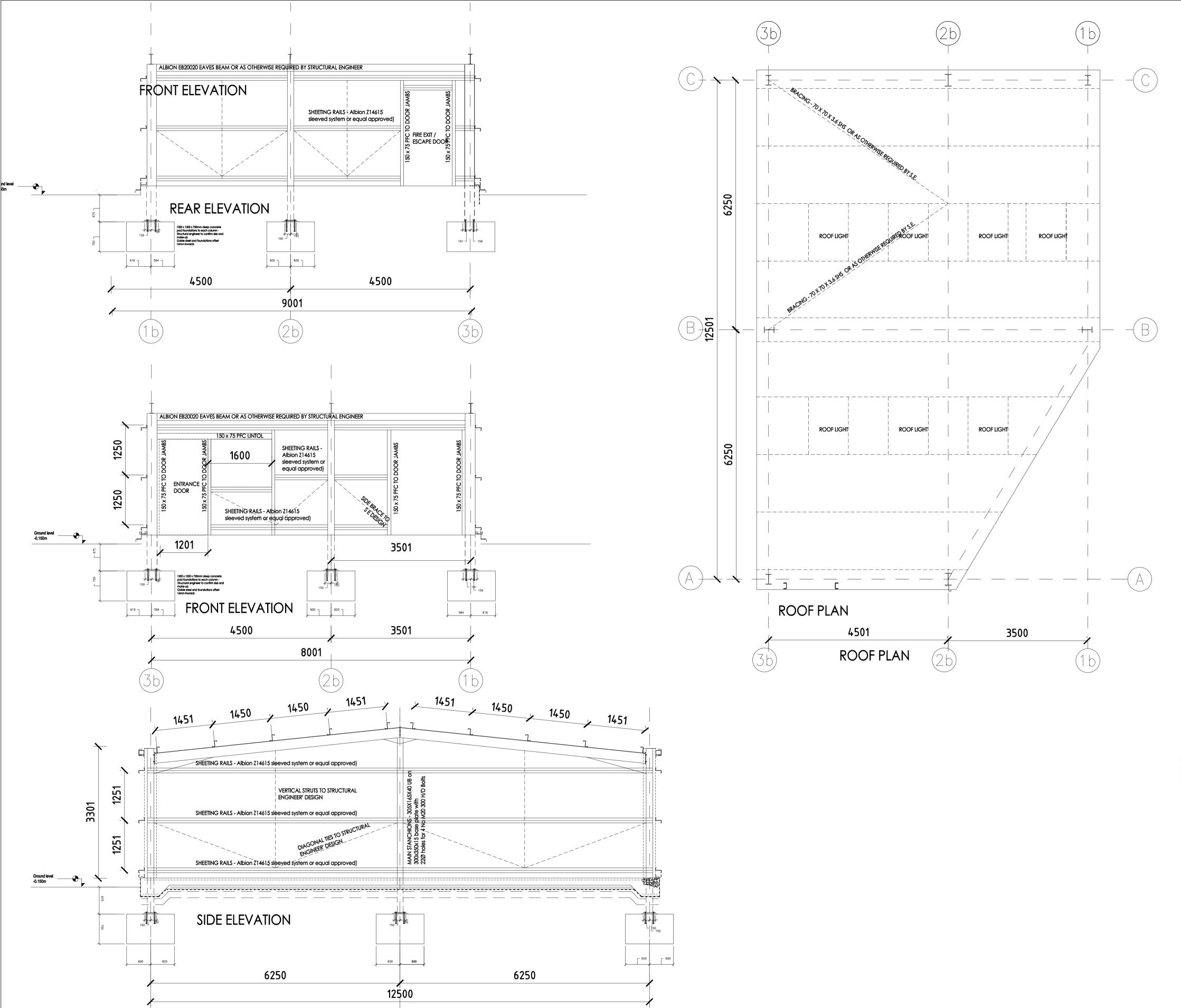
1200 X 1200 X 750mm deep mass concrEte pad foundations to each stanchion - all to Structural Engineer' specification and design Gable steel and foundations offset 16mm inwards
