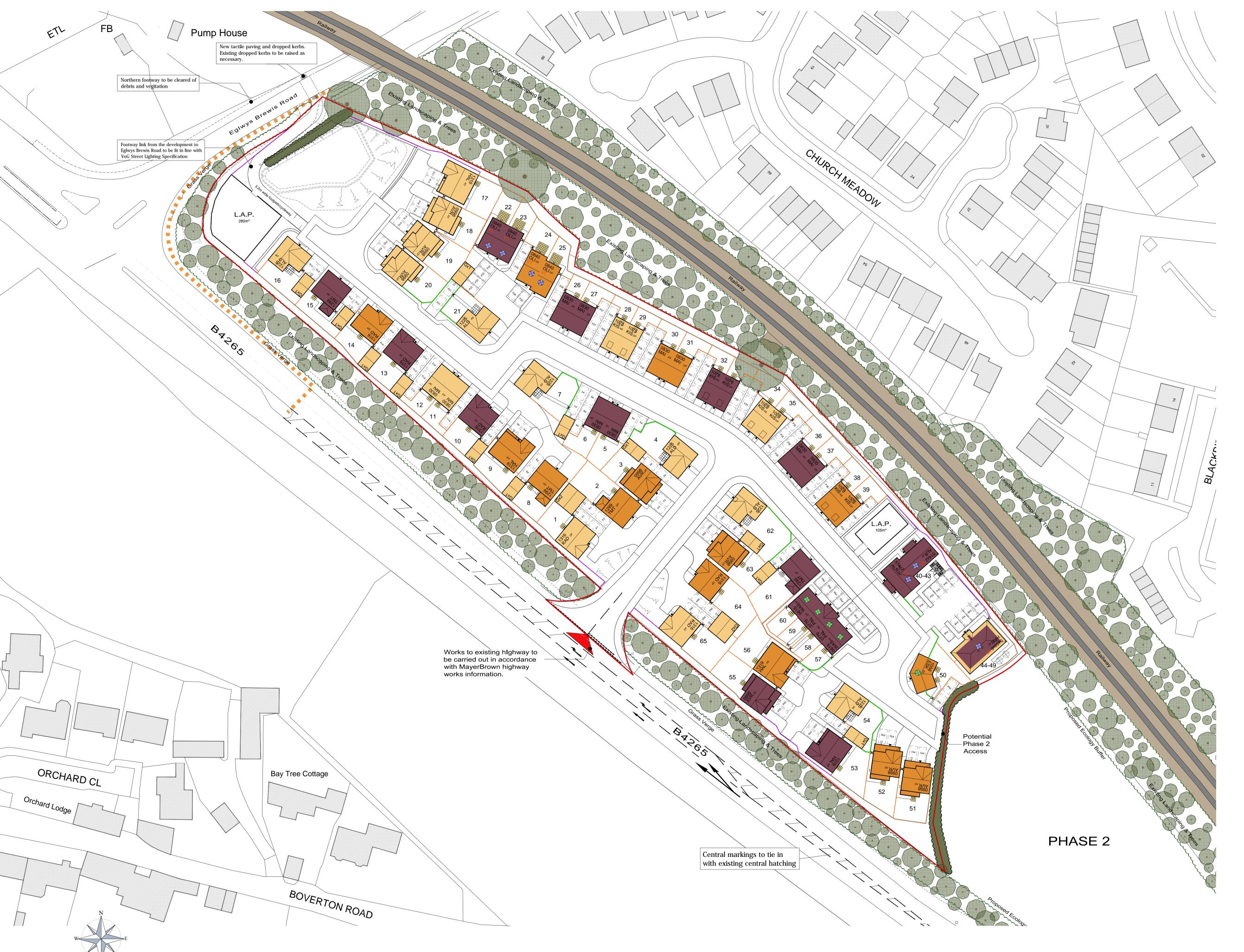
Site Key **Boundary Treatments** 1.8m High Timber Close Board Fence 2m High Close Board Fence with 130mm gaps at base for hedgehog movement 1.2m High Post and 3 Rail Fence 1.8m High Brick Screen Wall, Sunset Red Multi Proposed Hedgerow (refer to landscape architects drawings for further information) 1.8m High Close Board Gate **House External Finishes**
