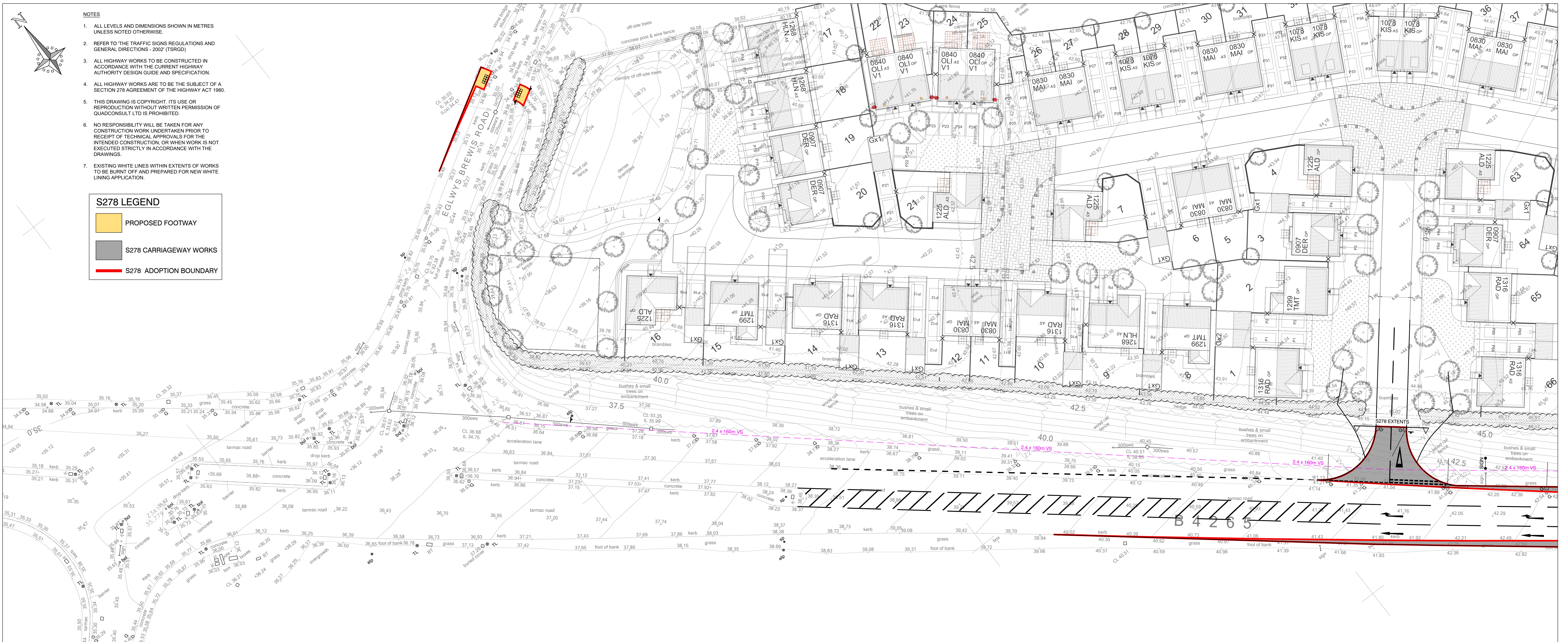
S278 GA - NORTH-WEST SECTION OF SITE SCALE 1:250
