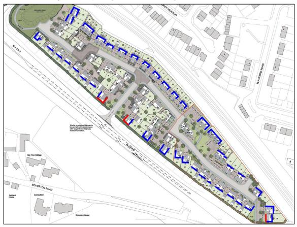
3309/SP2a – Façades Requiring Acoustic Glazing and Ventilation
