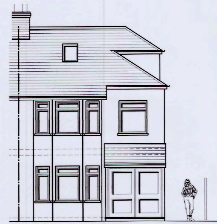
EXISTING FRONT ELEVATION - 1:100
