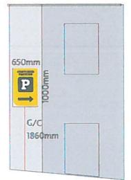
3mm White faced Aluminium composite with full colour vinyl graphic applied to face
