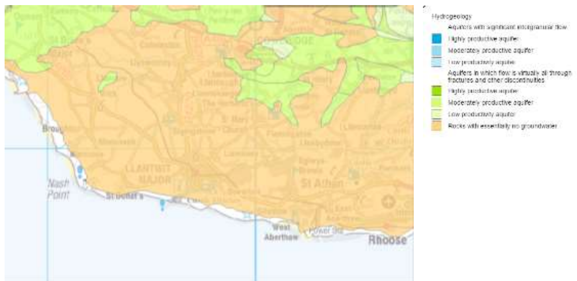
Figure 5: Map taken from the BGS, stating that the Jurassic Limestone has very little groundwater
